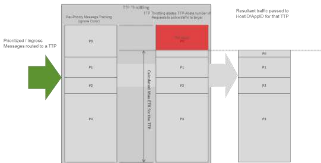
Figure 34 - Throttle by Message Priority Only when support for 5 message priorities is enabled
